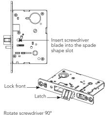
Rotate screwdriver 90° to push latch out until back of latch clears lock front, then rotate latch 180°, latch will then re-enter lockbody (NOTE: Latch can not be unscrewed)
