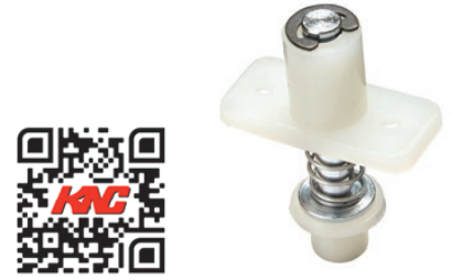
C-200B SPRING LOADED GUIDE Body 1-3/8" [34.9 mm] long x 5/8" [15.9 mm] wide Hole size required in door Ø 1/2" [12.7 mm] x 13/16" [20.6 mm] deep
