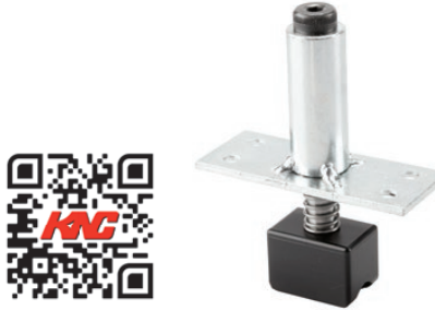
C-913SL SPRING LOADED GUIDE Plate 3" [76.2 mm] long x 1-1/4" [31.8 mm] wide Hole size required in door \varnothing 3/4" [19.1 mm] x MIN. 3" [76.2 mm] deep
